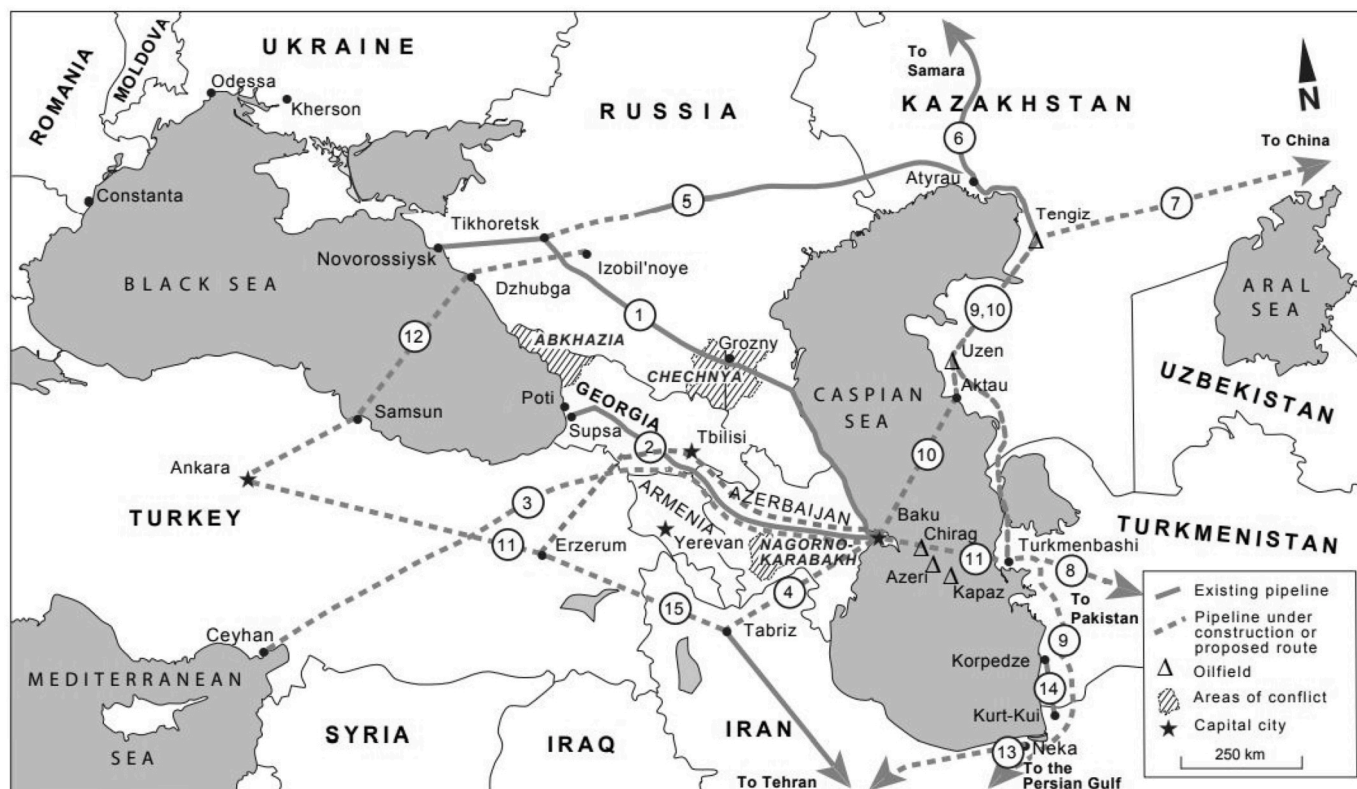
Fig. 4. Existing, under-construction, and proposed oil and gas pipelines in the Caspian region [61].
